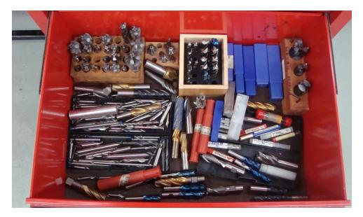
Here another drawer has been taken to show the current state of the end mill storage. This shows how poorly the current storage system is working and why it needs to be redone.
